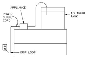
cord connecting an aquarium appliance to a receptacle. The "drip loop" is that part of the cord below the level of the receptacle, or the connector if an extension cord is used, to prevent water traveling along the cord and coming in contact with the receptacle. If the plug or receptacle does get wet, DON'T unplug the cord. Disconnect the fuse or circuit breaker that supplies power to the appliance. Then, unplug and examine for presence of water in the receptacle.
